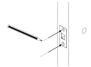
8 CHISEL UNTIL FACE PLATE FLUSH.
