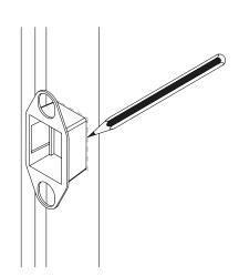
4 CHISEL UNTIL FACE PLATE FLUSH.
